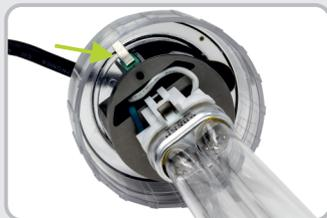
**IMPORTANT! NEVER** look directly at the UV light. Press and hold the small thin silver switch when the power is on and the bulb should ignite. Please test in a dark/ shadowed place and do not look directly at the bulb – we recommend covering the bulb with kitchen roll or similar. You should still be able to see the glow of the bulb through this.
