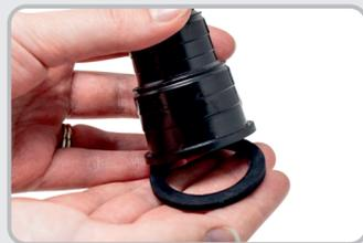
Make sure the O-rings are placed smooth side up to the hoesetail (see image on the right for reference). This will prevent leakage.
