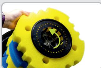
**Quartz sleeve & UV bulb** - remove the top part of the filter by unscrewing screws from the unit's head. Rotate the ballast in a clockwise direction and gently lift up the UV bulb.
