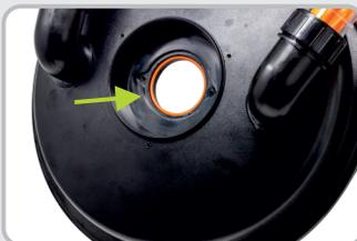
When reassembling your unit you must make sure the orange O-ring sits on top of the lid as seen in the image above. This will enable you to correctly reattach the quartz sleeve.
