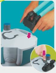
To attach the provided hoses to the filter, remove the hose adapter by lifting the hose adapter securing buckle and pulling the adapter out of the motor head. Install your hoses onto the Inlet and Outlet connections on the hose adapter and secure them into place using the plastic screw nuts. Push the hose adapter back into the motor head and re-fasten it using the securing buckle.
