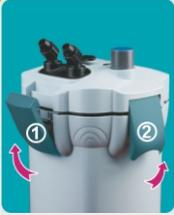
To open the unit, unfasten the 2 buckles that are situated at the front and back of the filter then lift the 2 levers that are attached to the left and right sides of the motor head. On doing this the motor head will lift away from the unit.
